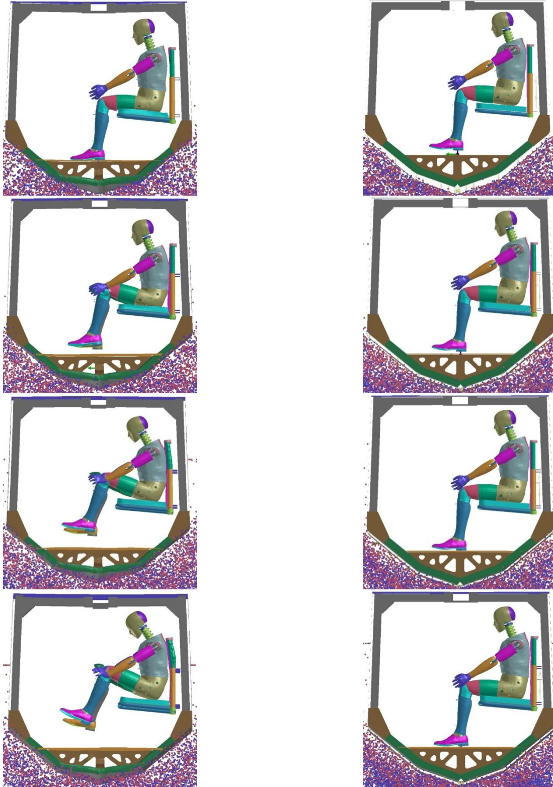
Figure 13: Occupant (ATD) response to blast in baseline case (left column) versus dual-hull (right column) at time points (from top to bottom) of 24 ms, 50 ms, 74 ms, and 100 ms.
